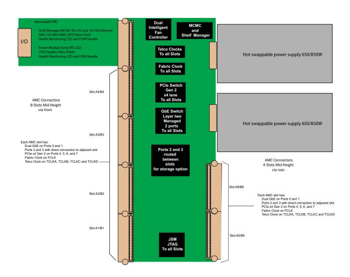
FIGURE 1. VT850 Functional Block Diagram
